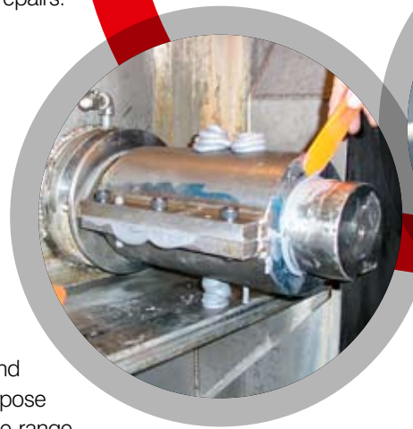
In-situ Shaft Forming
