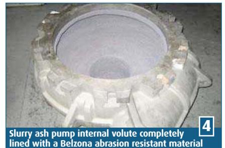
**4** Slurry ash pump internal volute completely lined with a Belzona abrasion resistant material
