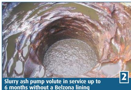
**2** Slurry ash pump volute in service up to 6 months without a Belzona lining
