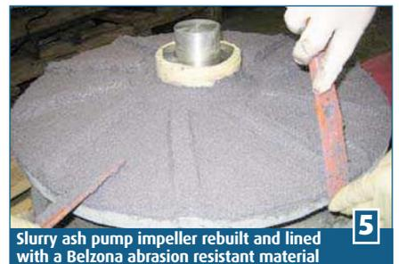
**5** Slurry ash pump impeller rebuilt and lined with a Belzona abrasion resistant material
