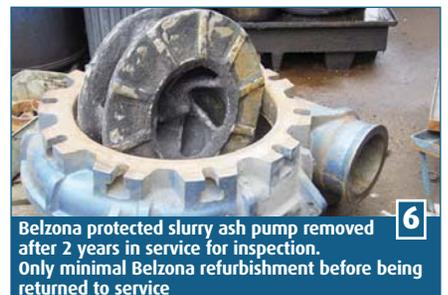
**6** Belzona protected slurry ash pump removed after 2 years in service for inspection. Only minimal Belzona refurbishment before being returned to service
