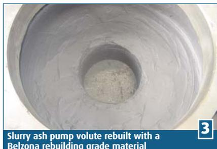
**3** Slurry ash pump volute rebuilt with a Belzona rebuilding grade material
