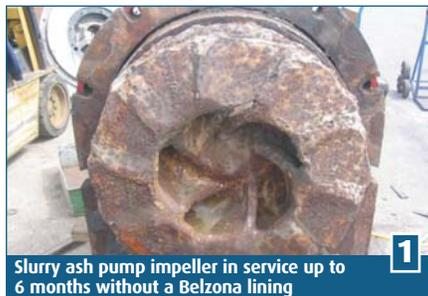
**1** Slurry ash pump impeller in service up to 6 months without a Belzona lining
