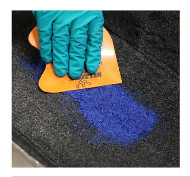
Belzona 1818 is a fast curing, surface tolerant, abrasion resistant system ideal for patch repairs on surfaces subject to high erosion and abrasive environments.
