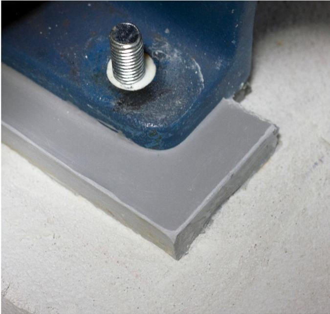
Belzona 7111 is a pourable chocking, backing and levelling system that has been developed to withstand the harsh physical and thermal shock of marine and industrial environments.
