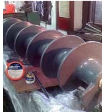
Screw conveyors protected
