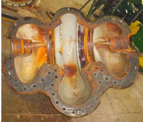
Fig 8: Belzona®1341 Supermetalgilde after 12 years service
