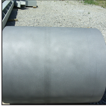
Surface preparation by blasting
