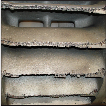
Main body of rotor severely eroded
