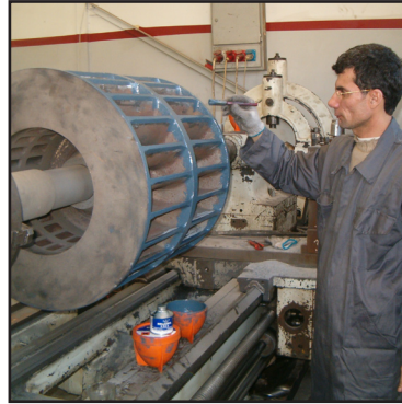
Top Coating with Belzona® 1321
