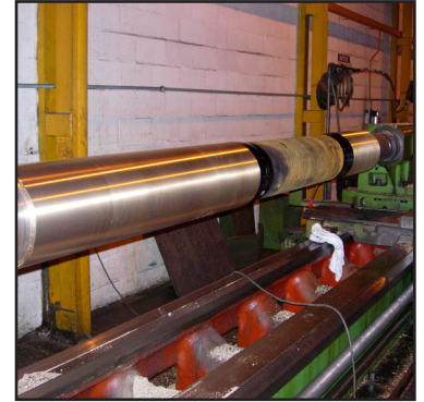
Tailshaft complete - all works were undertaken on the lathe
