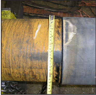
New liner fitted to shaft
