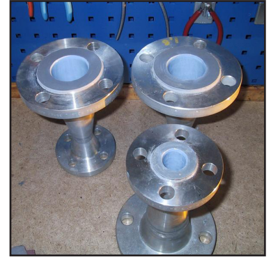
Individual small bore nozzle coating
