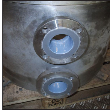
Exit nozzle coating
