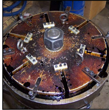
Mold fitted and filled, waiting cure
