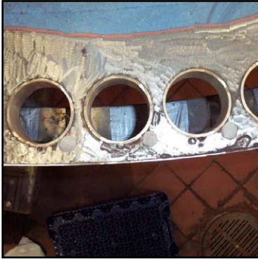
Bushings installed and table prepared. Note deep corrosion pitting
