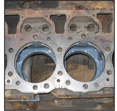
Applying Belzona® 1391 (Ceramic-HT) to the block
