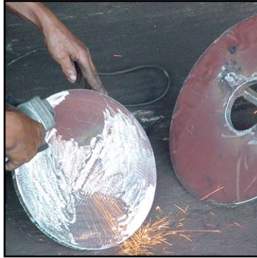
A 12" diameter plate is prepared with lifting hook.
