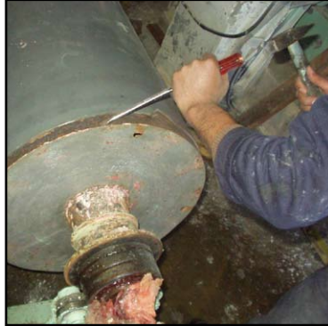
Removing the cracked layer
