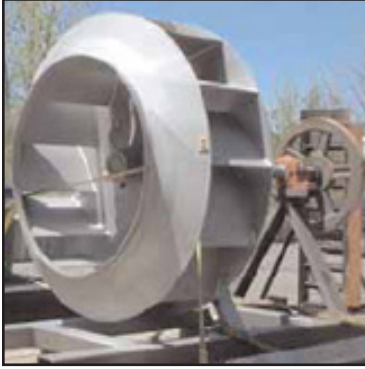
Fan blasted to 3-4 mil profile, white metal finish
