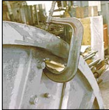
Knives C-clamped into the wet Belzona
