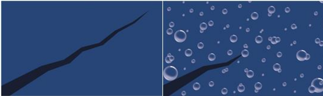
Crack propagation in other coatings (left) and Belzona 1523 and Belzona 1593 (right)
