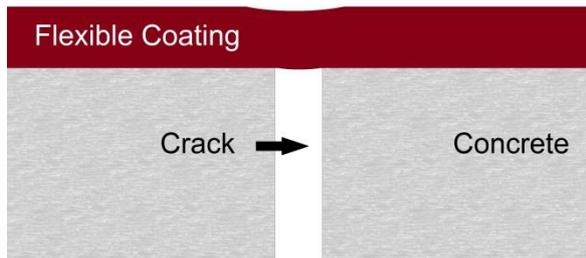
Fig 3 and 4 – Rigid vs flexible coatings
