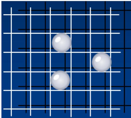
Fig 6 - Low crosslink density
