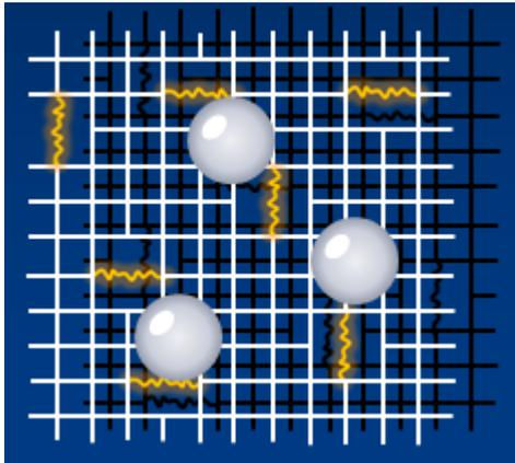
Fig 9 - Flexible segments in the polymer chain of Belzona 4361
