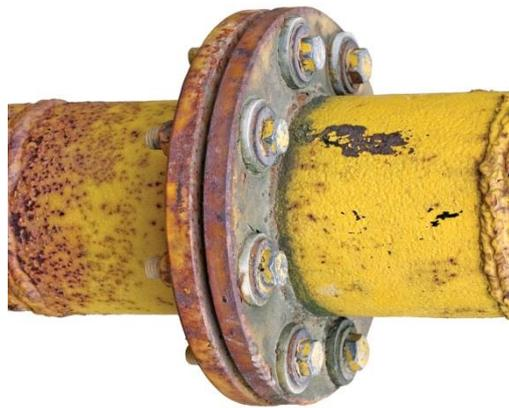
Figure 1. corroded flange
