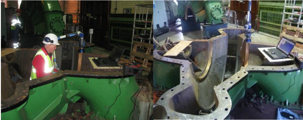
Image 4&5- Lower casing being scanned to capture hydraulic details
