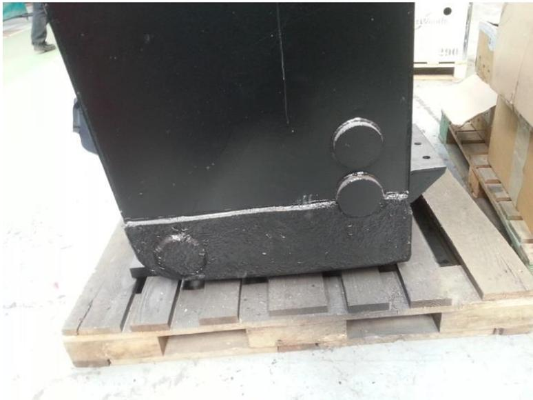
*Diesel tank restored using a cold-applied solution*
