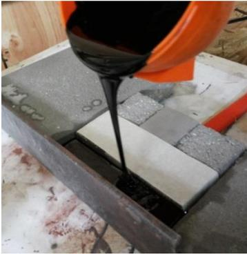
Pouring of flexible elastomer into sample piece
