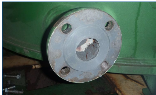
Flange face forming completed
