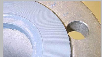
A flange face forming kit has now been made available and consists of necessary accessories to carry out flange forming applications. Currently available #300 psi, which includes six formers (2x2", 2x3", 2x4") covering all range of schedules.
