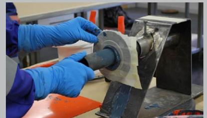
In conjunction with the flange face forming technology, vessels' weak points are effectively isolated from corrosive media.
