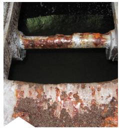
Pump casing severely corroded
