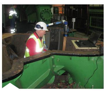
Lower casing being scanned to capture hydraulic details
