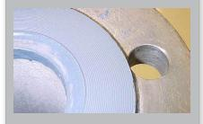
A flange face forming kit has now been made available and consists of necessary accessories to carry out flange forming applications. Currently available #300 psi, which includes six formers (2x2", 2x3", 2x4") covering all range of schedules.
