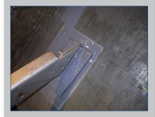
Belzona commissioned tests with Lloyd's register to measure tensile shear adhesion, tensile adhesion and cleavage adhesion of Belzona 1511 (Super HT-Metal) in March 2004. Tests were conducted using Schenk/Instron servo hydraulic test machine at 50% humidity and 23°C (73°F).
