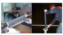
In order to protect small bore nozzles, a conventional coating would not be sufficient due to the risk of pinholes or holidays when coating a narrow nozzle. This issue is rectified by introducing prefabricated nozzles made from Belzona composites that do not corrode. The inserts and the nozzle are wetted out with a Belzona coating grade material, before being installed and bonded together to ensure corrosion protection.
