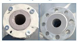
Flange face corrosion is a common problem affecting pressure vessels, where the face must be isolated to prevent oxidation. Belzona composite materials do not corrode and bond strongly to the flange face, where prefabricated formers are used to shape specified Belzona material on the flange face.
