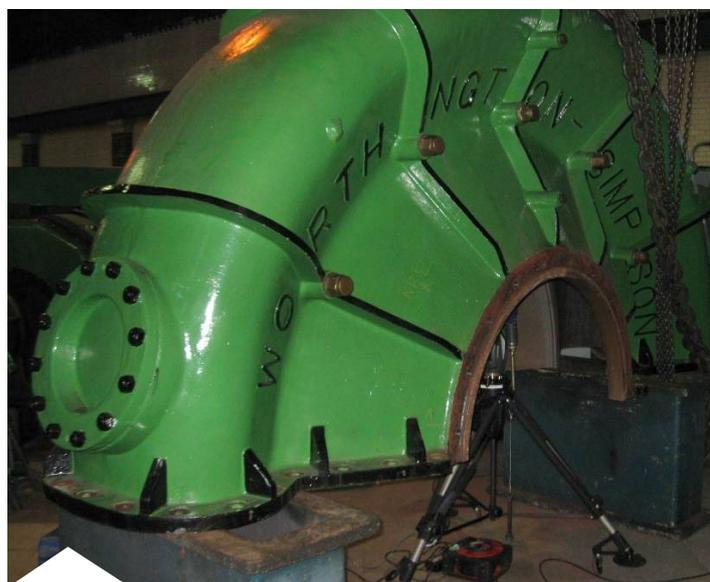
Pump casing mounted on blocks for screening
