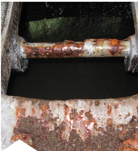
Pump casing severely corroded
