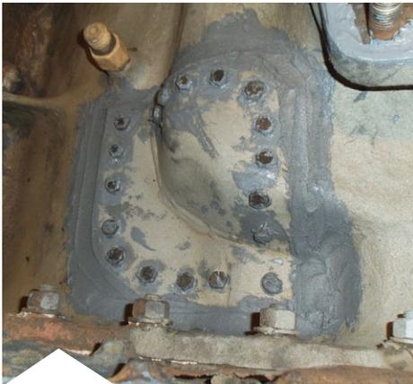
Plates bonded with epoxy repair composite
