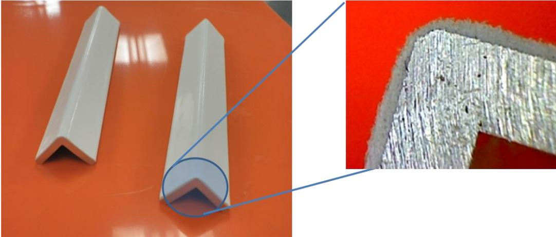
Figure 5: Excellent edge retention - NACE TM0304 specified 90° angle aluminium specimen with ridge radius curvature of 0.7mm. The peak to flat coating thickness ratio of 0.5 is achieved
