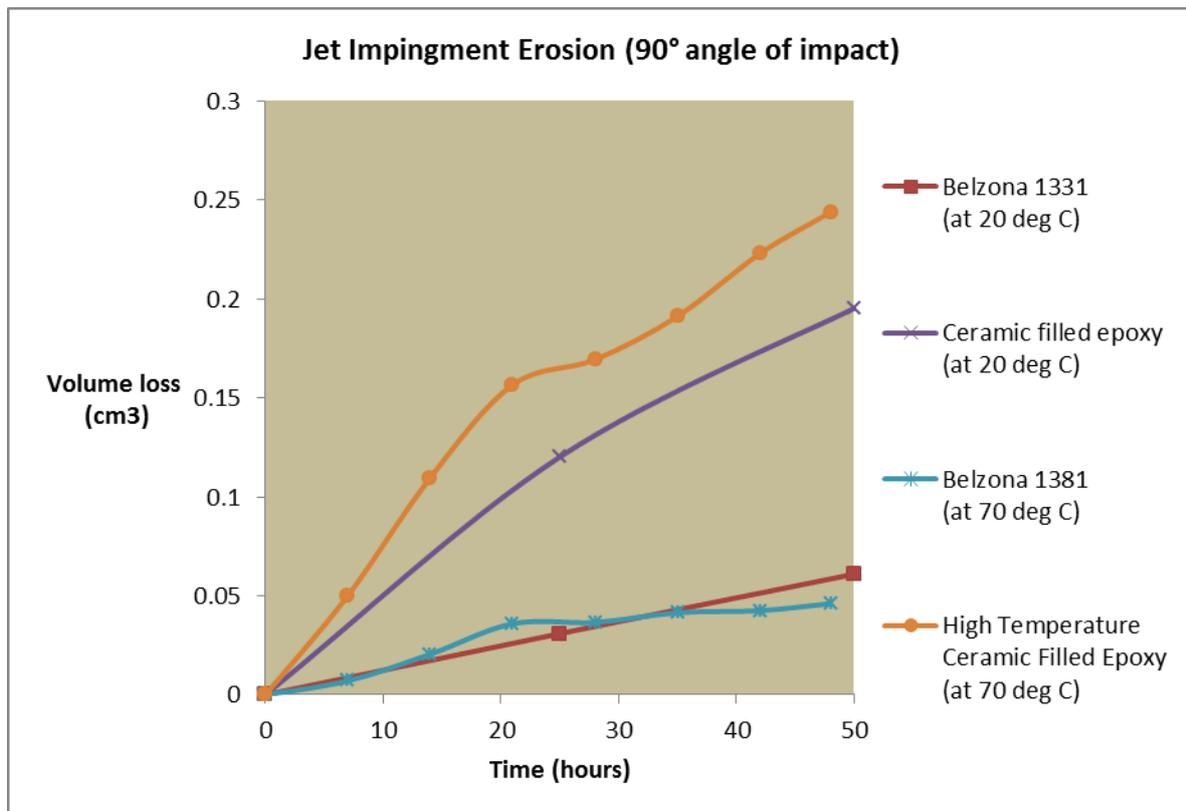
Figure 3: Belzona 1331 and 1381 jet impingement erosion versus ceramic filled epoxy coatings
