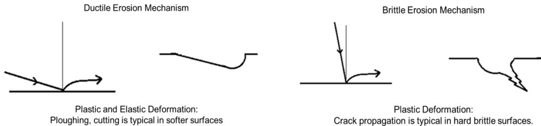
Figure 1: Diagrams of Ductile Erosion Mechanism and Brittle Erosion Mechanism demonstrate the mechanisms of erosion acting on a coating surface.
