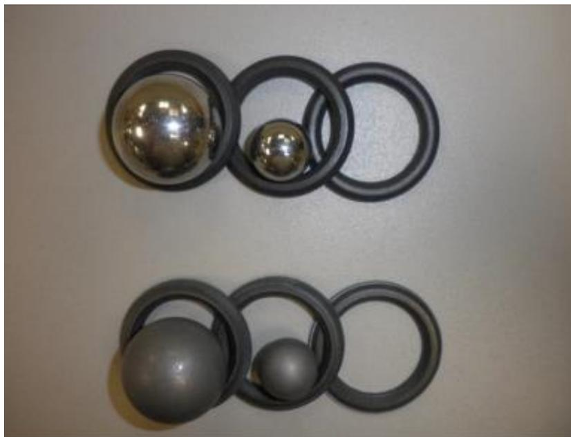
Figure 2: The packing seals and ball valves recovered from the piston exhibit a marked difference in the extent of wear resulting from the use of Belzona 1331 (top) and a 'sprayable' ceramic epoxy coating (bottom)
