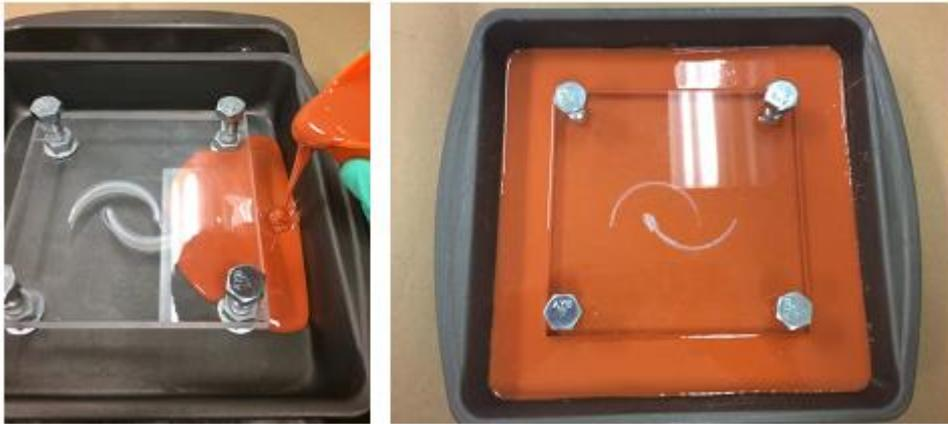
*Belzona 7111 application demonstration*
