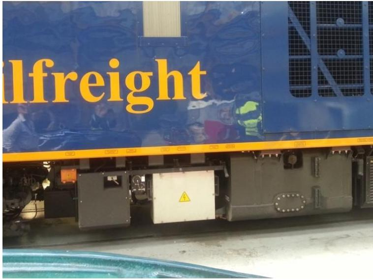
*Repaired diesel tank fitted onto refurbished train*
