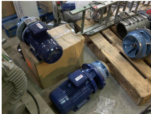
Impellers pre-coated with Belzona 1341 unpacked at the Stofnfiskur facility
