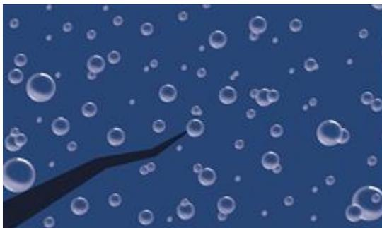
*The rubbery domains incorporated to Belzona 1523 and Belzona 1593 inhibit crack propagation*
