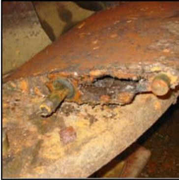
*Damaged Wicket Gate Blade.*
