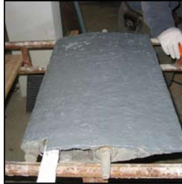
*Blade After Rebuilding With Belzona® 1111*
