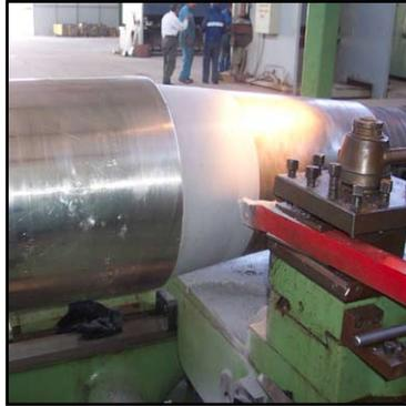
Rudder stock being machined back to its dimensions after repair.
