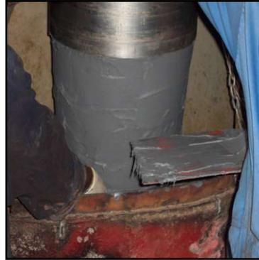
Belzona® 1121 was applied to both pintle and pintle housing.
