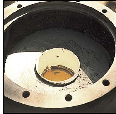
*Two coats of Belzona® 1321 (Ceramic S-Metal) applied.*
