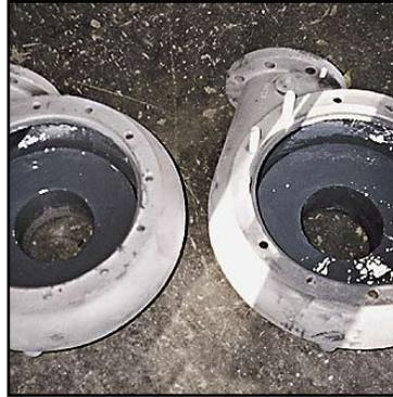
*Forming technique and Belzona® 1311 (Ceramic R-Metal) used to rebuild the intake.*
