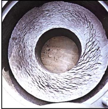
*Severe wear on the pump casing.*
