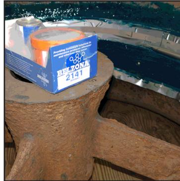
*Repaired surface rebated, taped, and half coated with Belzona® 2141*
